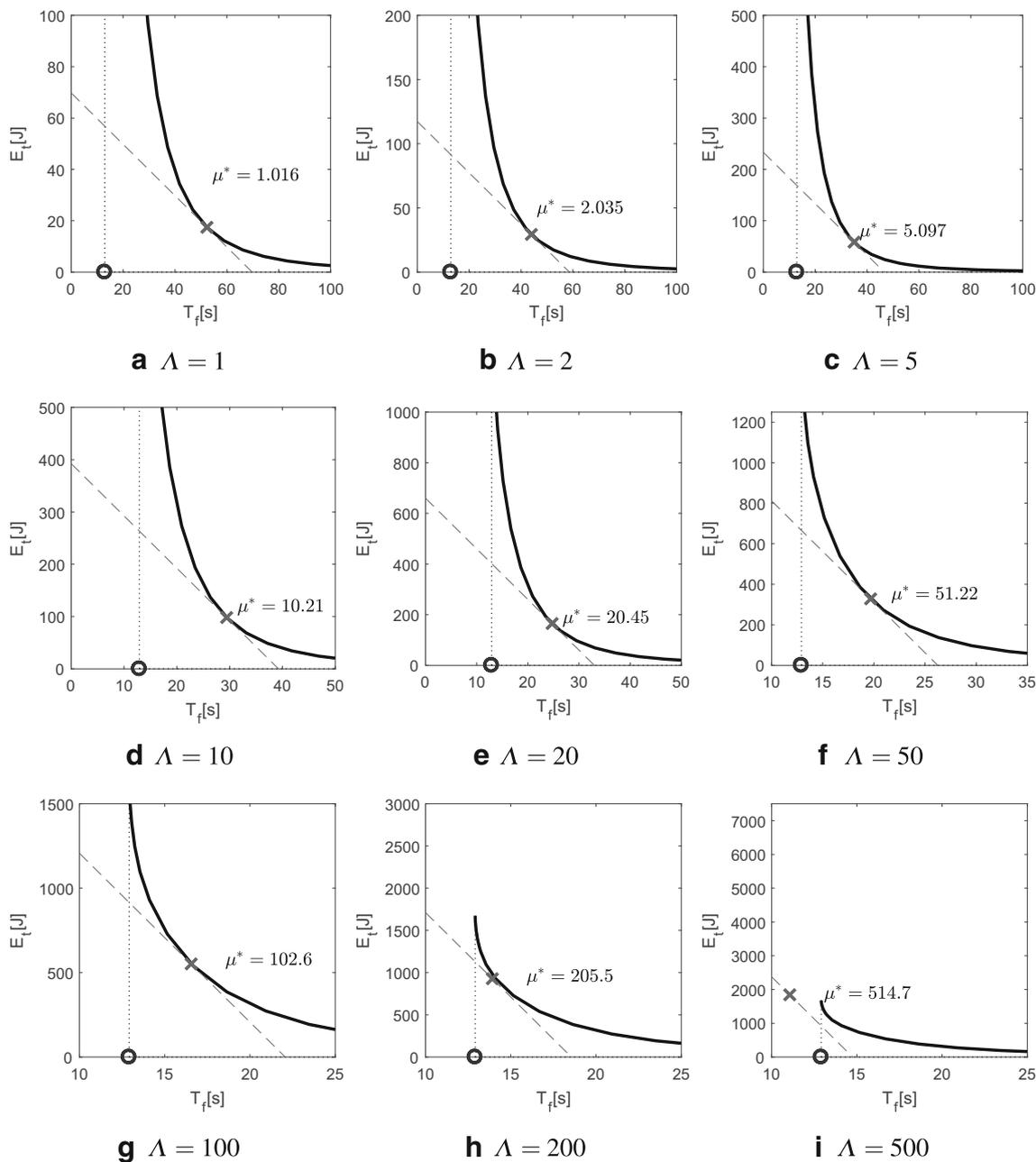
**Fig. 6** Criterion spaces  $T_f \times E_t$  in some tuning of  $\mu$  as function of  $\Lambda$ . The red cross indicates the Knee Point  $(T_f^*, E_t^*)$  calculated by the Algorithm 1 and the dashed red line represents the tangent of the Pareto Front at the Knee Point, with a slope of  $-\Lambda$
