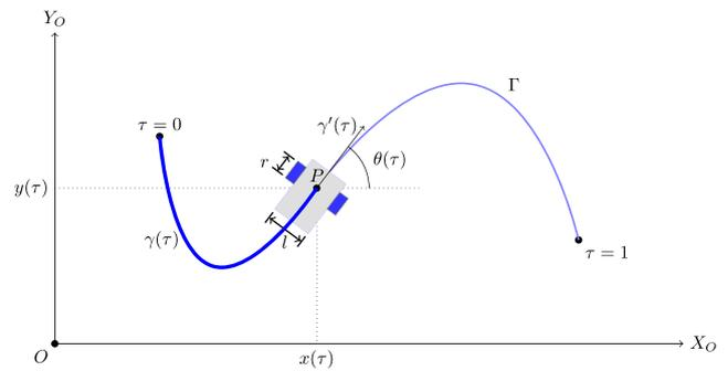
**Fig. 1** The WMR and its coordinates in two different representations, traversing a predefined geometric path  $\Gamma$  parameterized by  $\tau$
